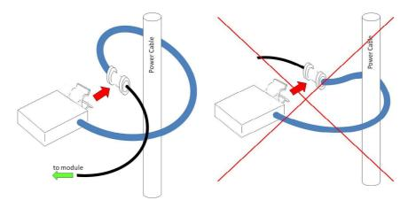
The sensor has to be properly aligned to the cable, as shown in the following figure.
